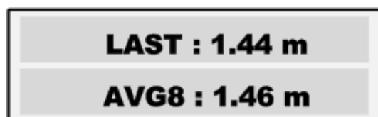
Figure 9: Example LCD display showing last and average range
