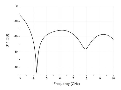
Figure 5 Antenna match versus frequency
