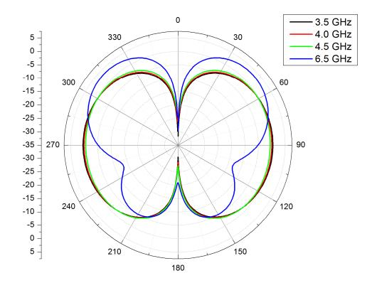
Figure 4 Radiation Patterns Elevation (phi 0°)
