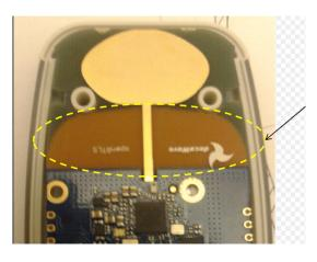
By incorporating part of the antenna ground plane into the rest of the ground-filled PCB design, the overall size of a tag can be reduced.
