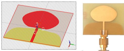
Figure 1 WB002 antenna, graphic and photo
