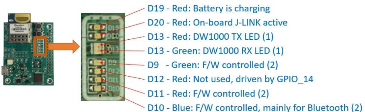
Figure 2: Front View of the DWM1001-DEV Module Development Board
