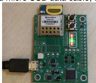
Figure 6 DWM1001 DEV board – micro USB connection
