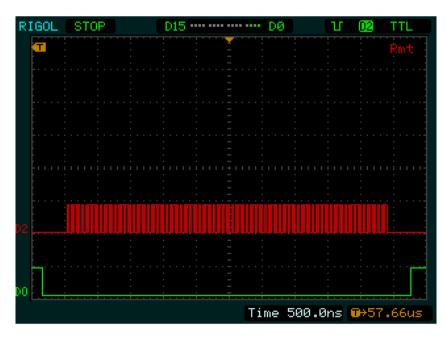
Figure 2: 18MHz SPI transaction using Cortex M3 with DMA
