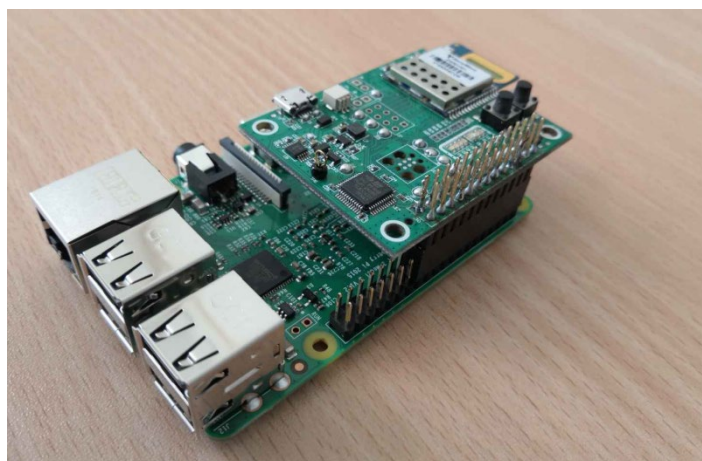
Figure 10: Gateway: R3B plus bridge node (DWM1001-DEV)
